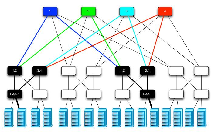
Insert flow entries to use multiple path through network Support multiple virtual networks (multiple tenants) Adjust flow entries when VMs migrate (move network with VMs)
